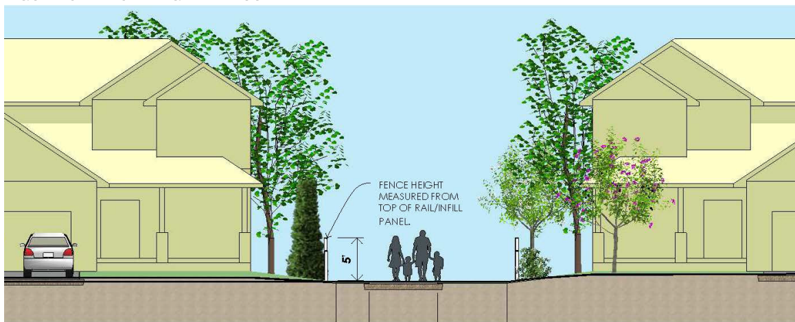
FIGURE 7. EXAMPLE: FENCE STEPPING DOWN WITH GRADE
