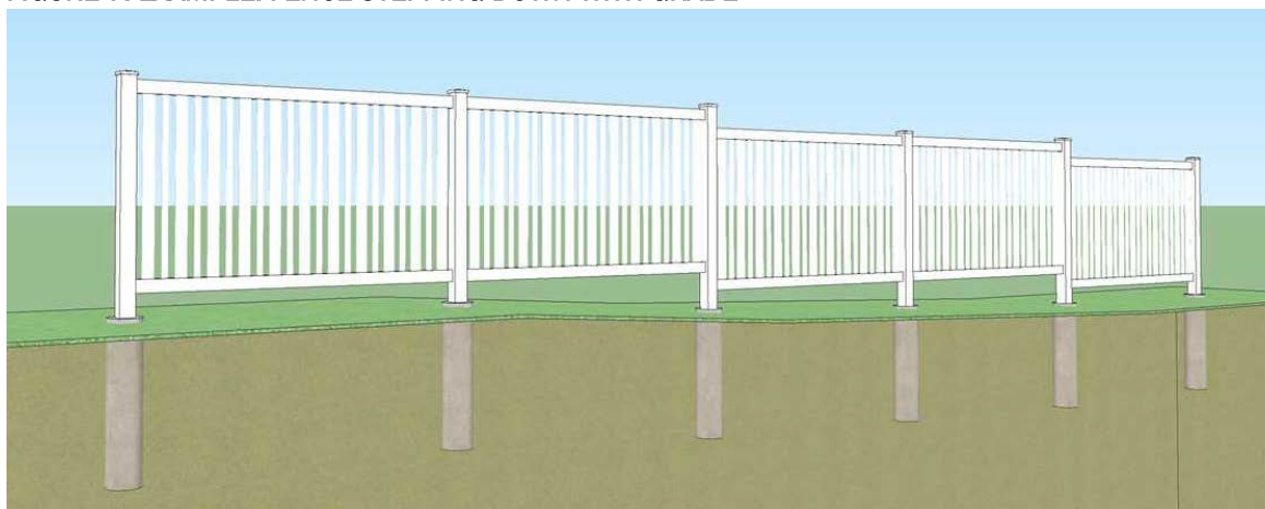
FIGURE 7. EXAMPLE: FENCE STEPPING DOWN WITH GRADE
